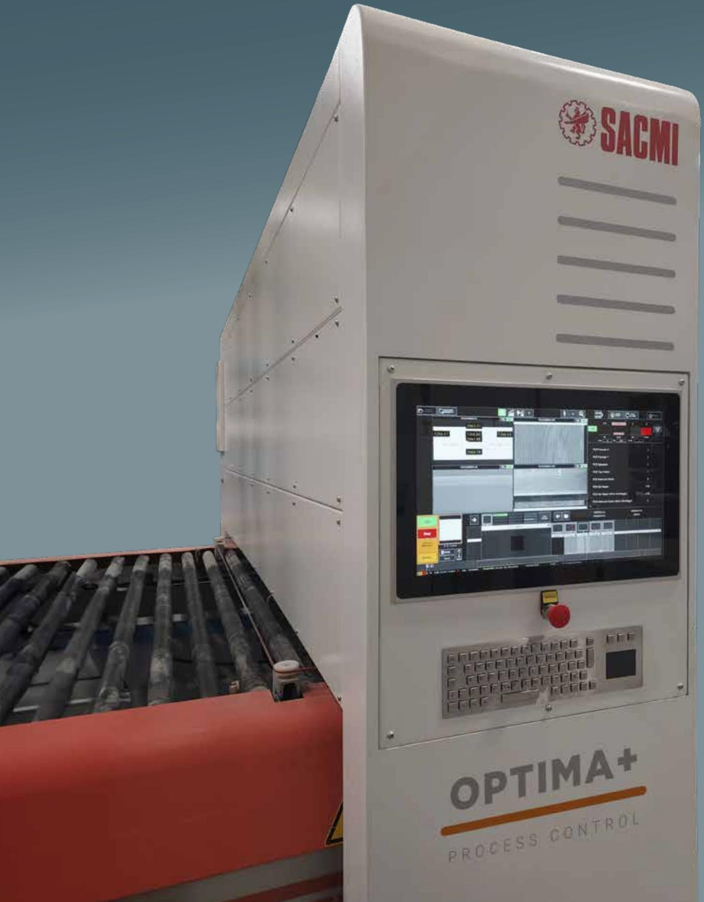
Optima+ was created to ensure impeccable quality. Using a non-invasive analysis, it examines each piece, instantly discarding slabs with surface or edge imperfections (small cracks or laminations). Inspection takes place before the slabs undergo further processing, thus optimising the process.
