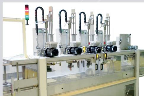
Enclosed polishing space with overhead polishing spindles
